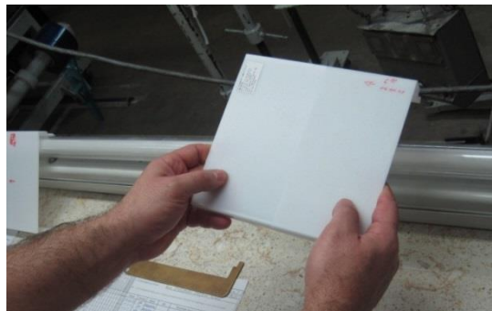
Figure 7: Top view test in incident light; Work lamp (transmission) is switched off
