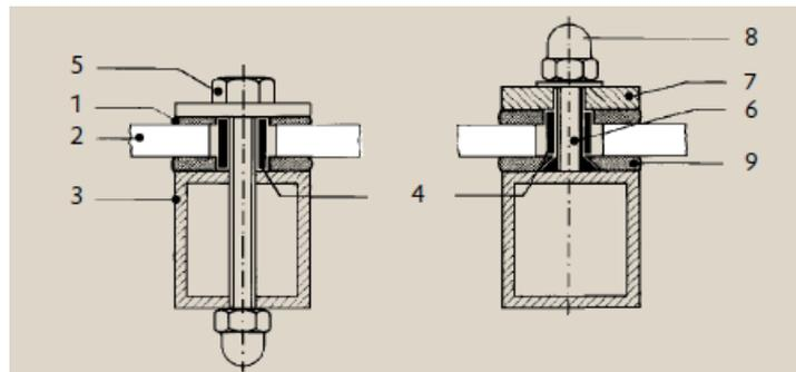
Self-tapping screws, which penetrate only into the plastic, are not suitable. However, they can be used if the thread is in contact with a metal counterpart and through holes are provided in the plastic (see above). In addition, the head of the self-tapping screw as well as the washer must be large enough as described above.
