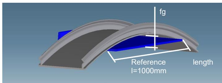
**Figure 5: Y-direction straightness**
