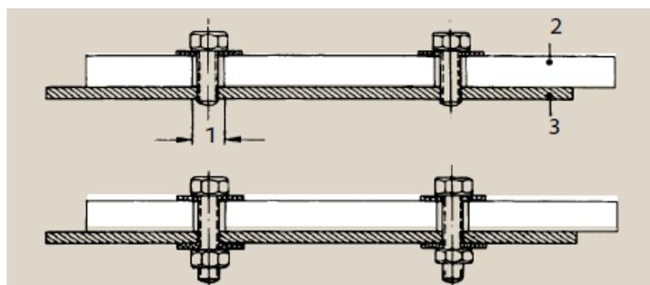
The clamping forces acting on the plastic part decrease with falling temperatures and increase with rising temperatures. This effect can be compensated by the use of washers made of EPDM, PE, PTFE (non-plasticized PVC!), etc. (see figure below).
