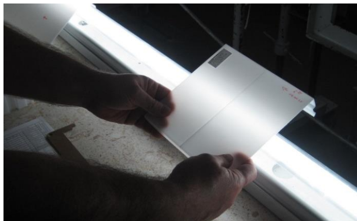
Figure 8: Visual inspection in transmitted light
